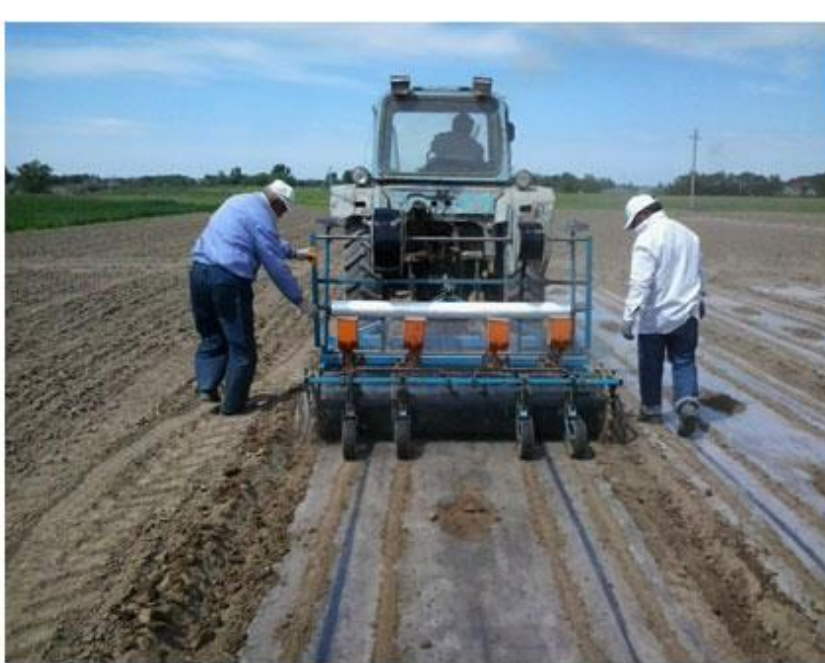
Figure 3 – Double-row rice sowing with laying of both irrigation tape and tensioning of the film
